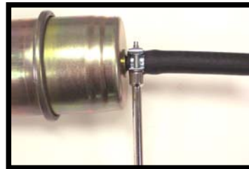
Proper Clamp Installation
