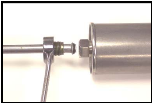
GM Threaded Fitting Removal
